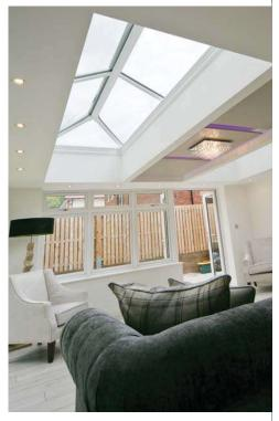
The Ultrasky Lantern can be inserted into a flat roof or a traditional orangery deck and is ideal for large builds where the roof height is restricted. Unlike many other lanterns, Ultrasky Lantern has a 25° pitch which draws more light into the room creating a stunning focal point.
