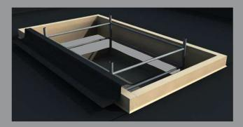
A timber kerb of 150mm high  $\times$  70mm wide (not supplied) must be fitted around the opening in the flat roof – the weatherproofing membrane laps onto the top face of the kerb.
